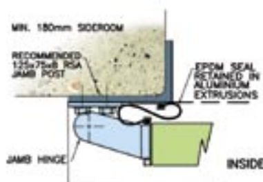
TYPICAL JAMB DETAIL
